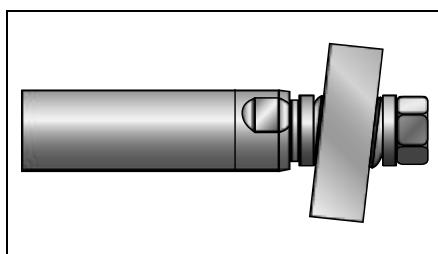
Mounted payload with radial and angle offset.
