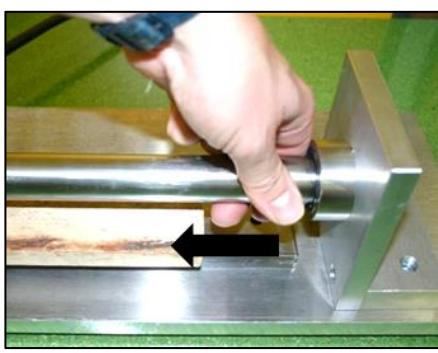
3. Put a spacer (wood, plastic, aluminium with thickness 15 mm) between slider and linear guide. The spacer prevents injuries to the hands and damage to the slider surface!
