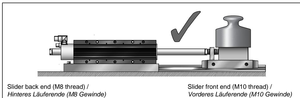
When attaching the load, the wrench for tightening the load must be used only on the load-facing side of the slider. Avoid torsional stress on slider (note the following figures).
