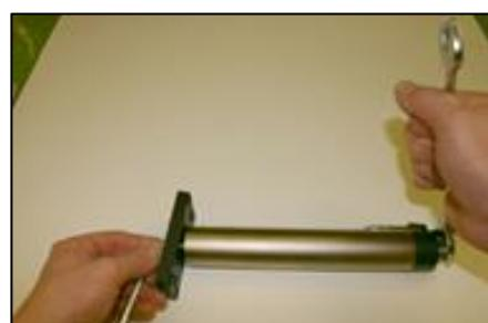
Incorrect attachment -> Torsional stress on slider
