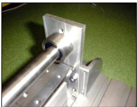
5. Place the floating bearing on the slider and attach to its support – **do not tighten the screws**.
