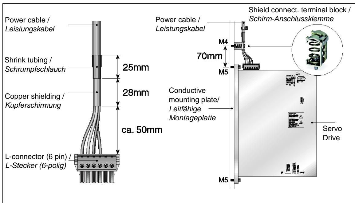
The power cable is supplied with a copper shielding (see illustration above). This prevents electrical and / or magnetic fields.
