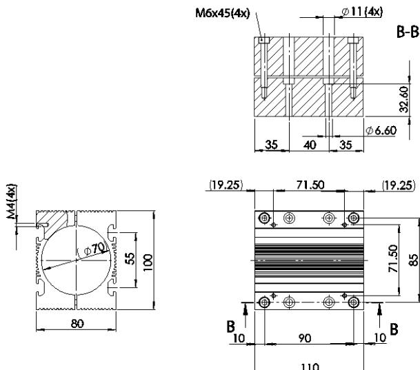
Max torque for clamp plate screws: 12 Nm (8.85 lbf ft)
