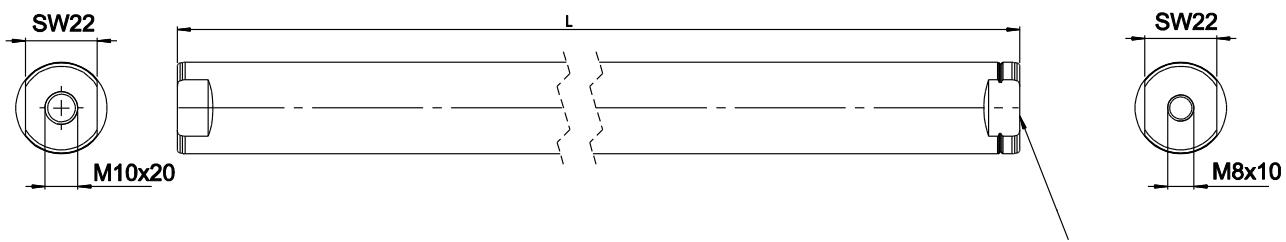
Slider front end M 10 thread
