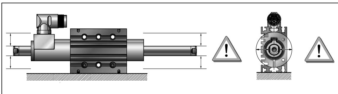
When installing linear motors in modules with metal parts near the slider, undesired forces can arise due to magnetic attraction or eddy currents. These generally manifest as erratic and jerky positioning, or reduced dynamics of the linear motor.
