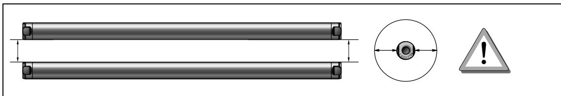
The sliders are made of neodymium magnets and have a strong magnetic attraction. It must be kept a minimum distance between the sliders. This minimized the risk of bruising and secondly, the sliders do not influence each other through their magnetic fields.
