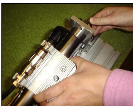
7. Move stator (front side) to the floating bearing and tighten screws
