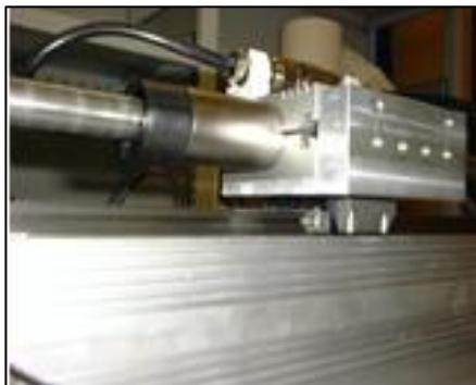
1. Mount stator to its support bearing
