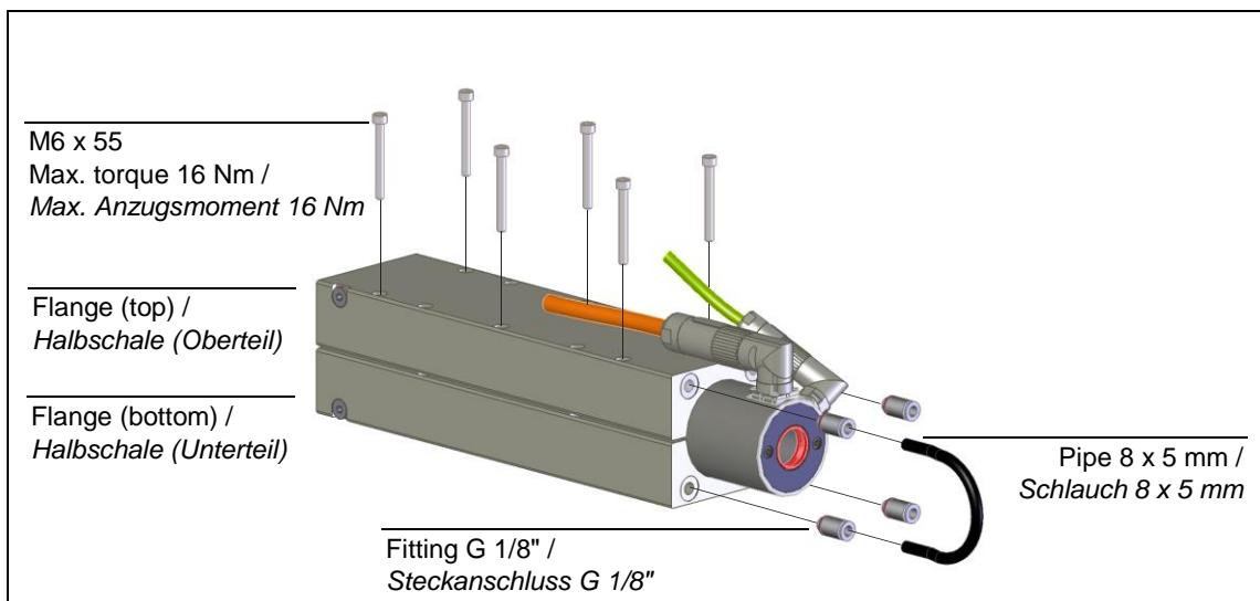
The fluid cooling flange consists of two half-shells. In both half-shells, a channel is incorporated, in which the cooling water can circulate in longitudinal direction. Via an external pipe connection, the channels of the two half-shells are connected in series.
