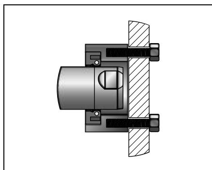
Floating bearing assembly that permits radial adjustment of slider position and permits a small amount of radial and axial movement.
