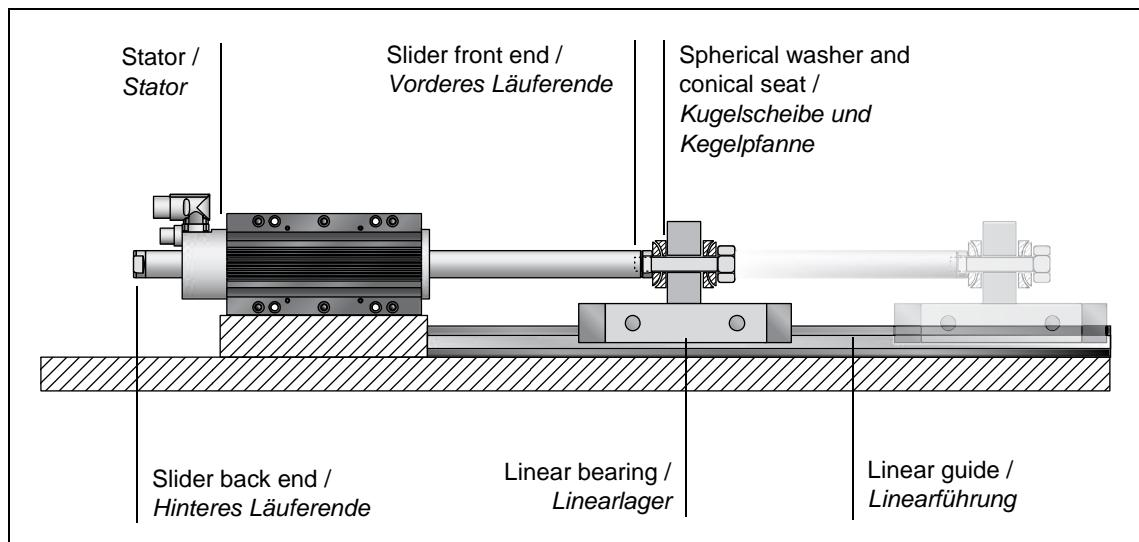
In a "moving slider" installation, the stator is fixed and the slider is the moving part. The load, borne by a linear guide, is attached directly to the end of the slider. In order to compensate for misalignment, spherical axial bearings consisting of spherical washers and conical seats (see the section 6.7 Slider mounting kits) are used to connect to the load. The mounting kit of slider and an oversized hole for the screw make it possible to adjust a radial and angle offset.
