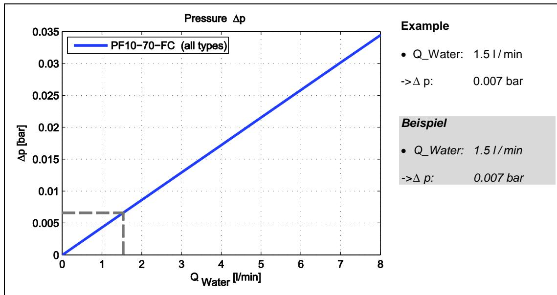
The required water pressure to inject the required water flow depends on the hydraulic resistance of the cooling circuit.
