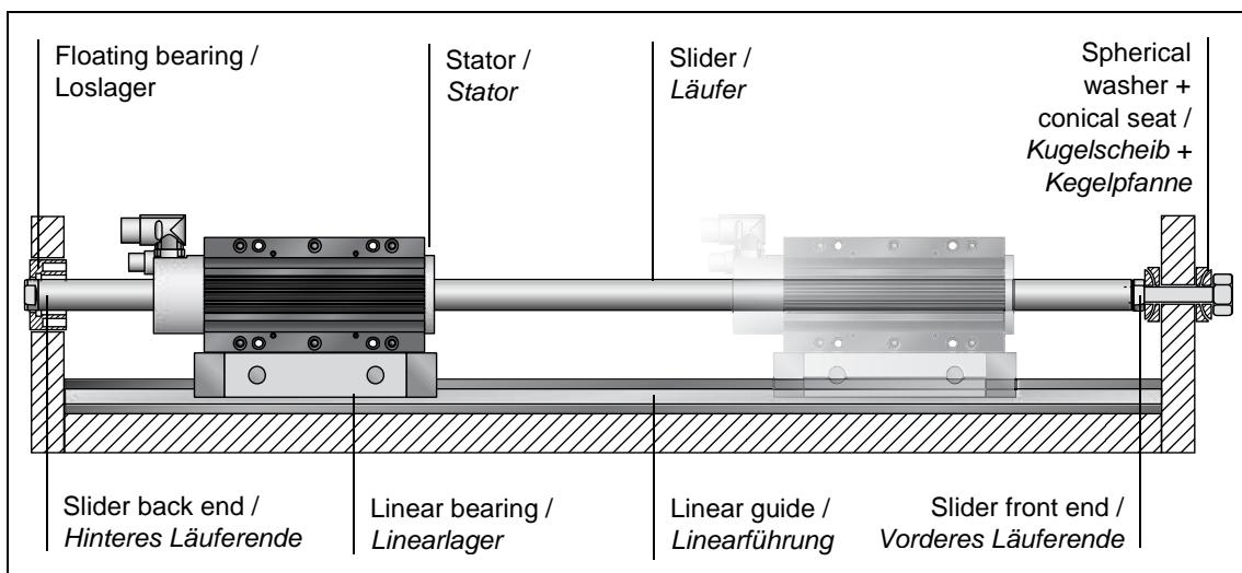
In "moving stator" applications, the slider is fixed and the stator is the moving part. The load is attached to the stator, which is mounted on a linear guide. In order to avoid an overconstrained bearing mount and compensate for alignment errors, the slider may be mounted on one end in a fixed bearing with a spherical axial bearing. On the opposite end, the slider is mounted in a floating bearing. Mounting kits are available for mounting the slider (see the section 6.7 Slider mounting kits).
