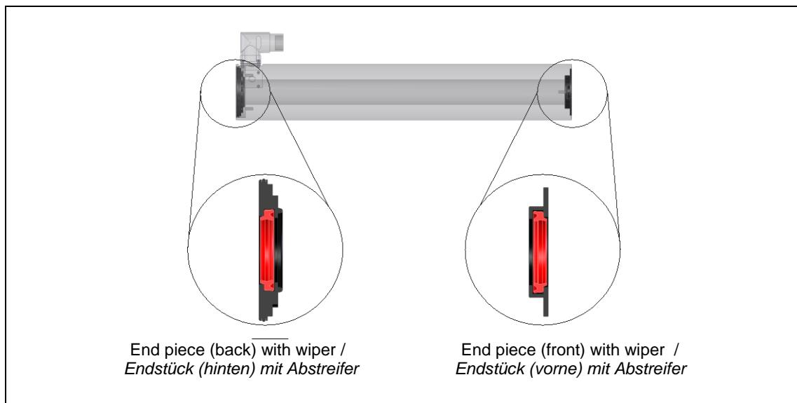
The stators are equipped as standard with wipers. This simplifies maintenance and the maintenance cycles can be extended. The wiper effects that the lubricant is dispensed metered and does not leak outside of the stator. The lubricant is less dirty.
