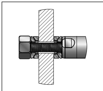
Slider mounting kit consists of a spring washer, a pair of spherical washers, and a pair of conical seats. It allows the slider to be fixed in the direction of motion. It also helps to compensate for radial and angle offset.
