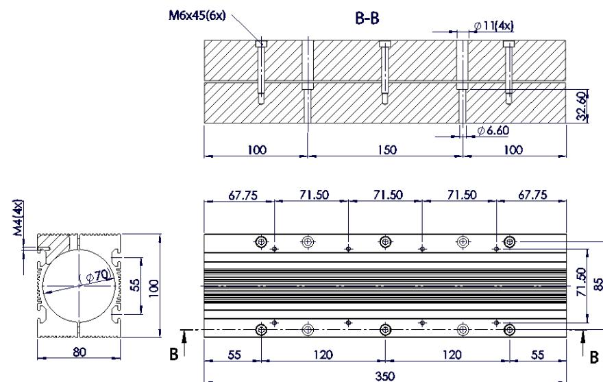
Max torque for clamp plate screws: 12 Nm (8.85 lbf ft)
