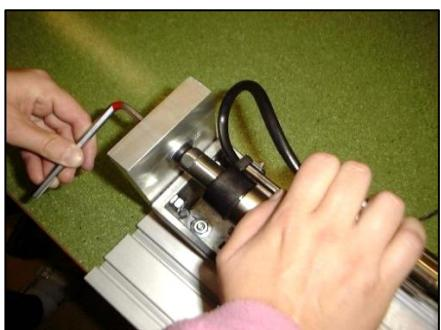
6. Move stator (back end) to the fixed end of slider, center slider in stator and tighten the screw.
