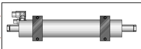
Incorrect mounting -> Small contact area prevents cooling of the linear motor.
