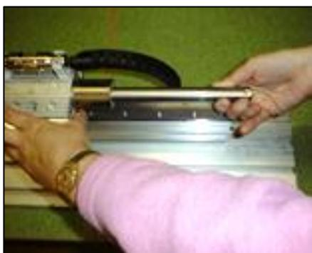
2. Insert slider into stator
