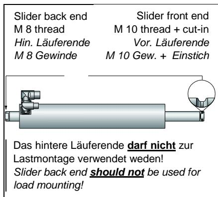
**4. Checking the installed direction of slider:**
