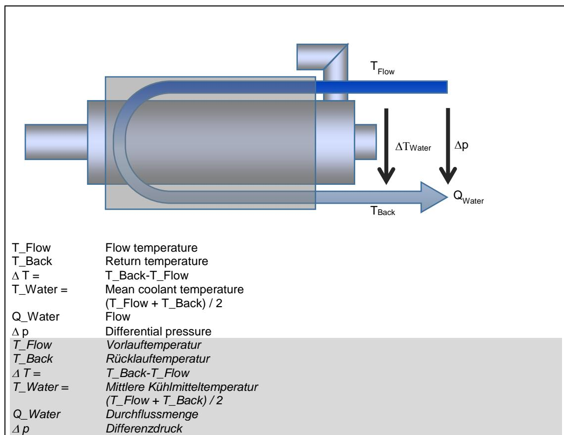
With the water cooling, the coolant is passed through the cooling circuit of the motor flange. Starting from the adjusted mean coolant temperature  $T_{Water}$  all other parameters of the cooling circuit may be dimensioned based on the diagrams referred to:
