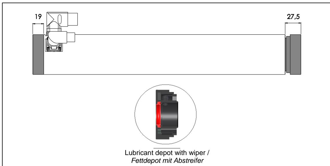
If the stators are equipped with lubricant depot, lubrication can be optimally regulated. It releases only as much lubricant as necessary. The maintenance is simplified and maintenance cycles are extended.
