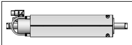
Forced cooling with fluid cooling flange to increase the continuous force. More details in chapter 4 Fluid cooling.
