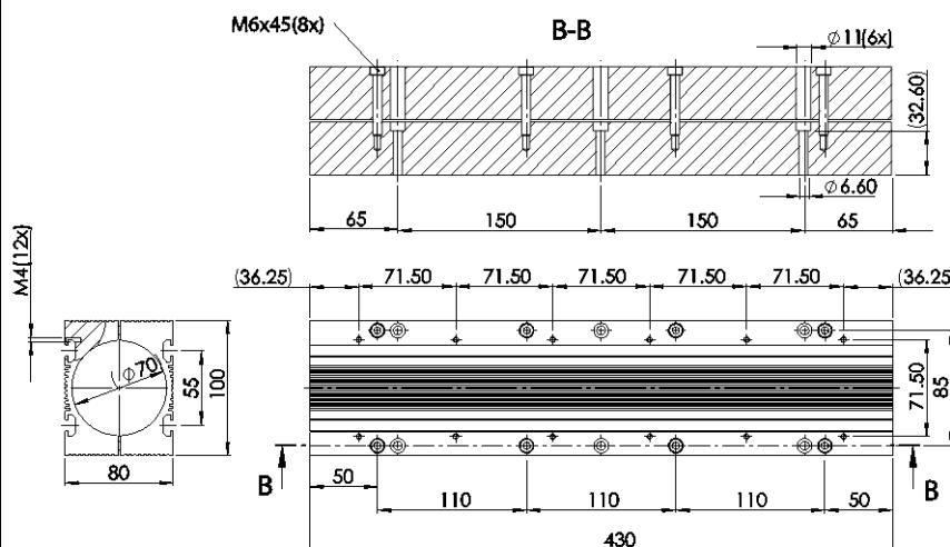
Max torque for clamp plate screws: 12 Nm (8.85 lbf ft)
