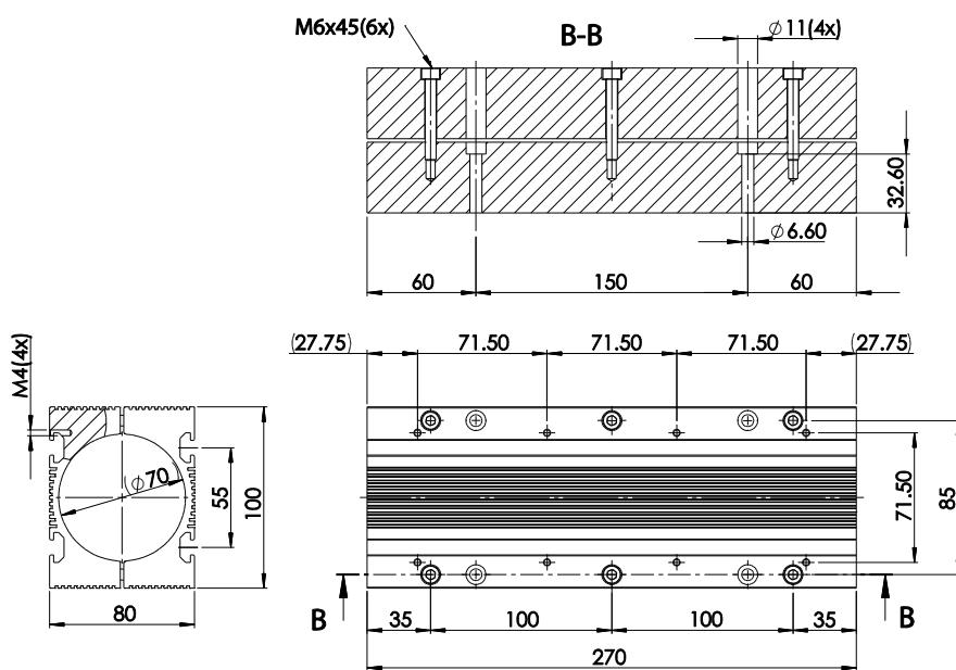
Max torque for clamp plate screws: 12 Nm (8.85 lbf ft)
