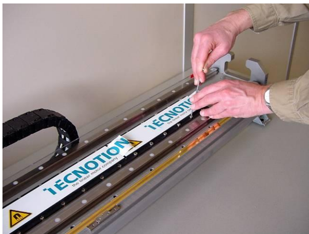
Figure 7: Installing a linear motor system
