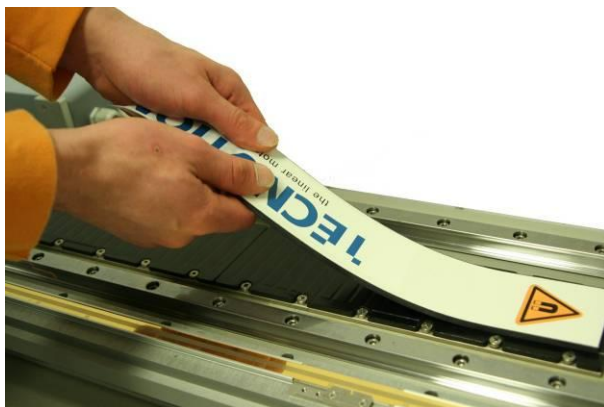
Figure 16: Uncovering the magnet track
