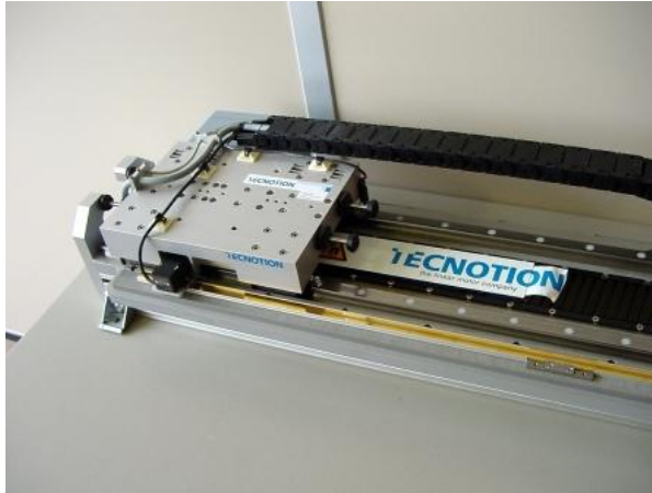
Figure 14: Securing the slide with a protection plate
