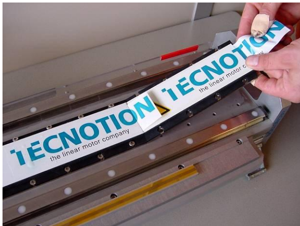
Figure 15: Placing another magnet plate
