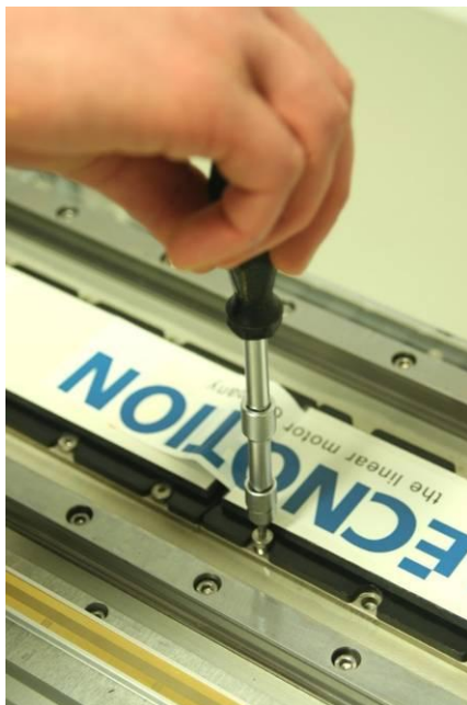
Figure 13: Mounting the Magnet plates
