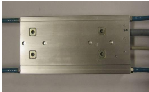
Figure 24: TL-water-cooling with four connection points
