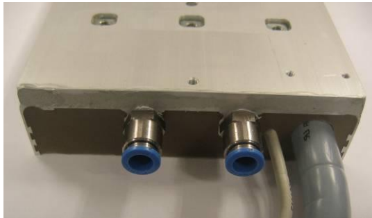
Figure 23: TBW-water-cooling with two fittings
